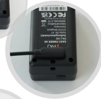
2. Connect the other end of the charging cable to the USB port of the wall plug adapter.
