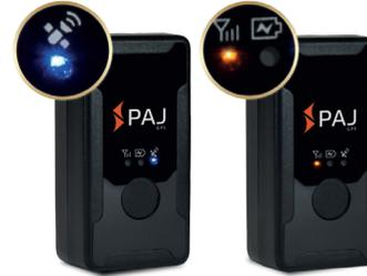
The LEDs flash alternately for 12 seconds
