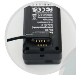
1. Connect the supplied charging cable with the magnet to the contacts of the FINDER.
